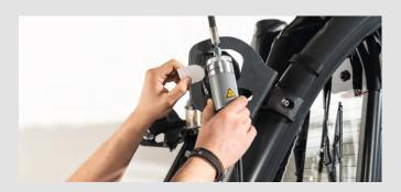
Formation of condensate while measuring soot is avoided by heating. The specifically required exhaust volume is ensured by regulating the gas pump.
