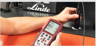
For determining the optical density (Bosch smoke number) the NOVAplus FFZ comes with a densitometer, which exactly determines the smoke number.
