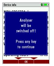
During a measurement or a battery charging cycle the auto off is deactivated.
